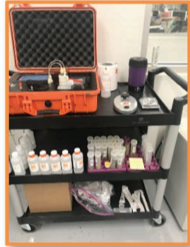
Figure 2. Example of mobile chromatography system (permission of Light Lab, Orange Photonics).
