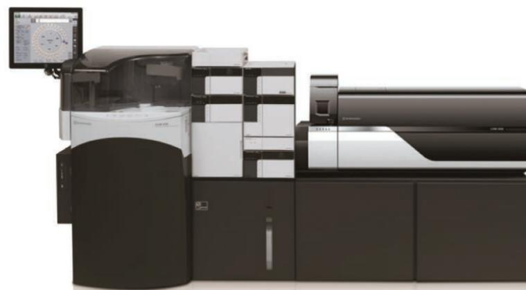
Figure 1: General view of the LC-MS/MS system with integrated sample preparation module CLAM-2000.
