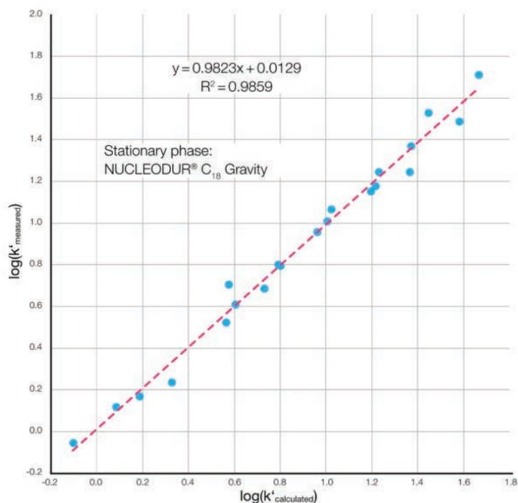
Figure 1: Plot of  $\log(k'_{\text{measured}})$  versus  $\log(k'_{\text{calculated}})$
