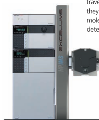
Figure 1. The IA3100 HPLC-HPIMS system from Excellims Corporation. The HPLC module on the left (courtesy of Shimadzu Corporation) includes autosampler, column, and pumps. The HPIMS on the right includes an ESI source, drift tube, and Faraday plate detector.
