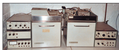
Figure 1. Pye 104 Gas Chromatograph.
