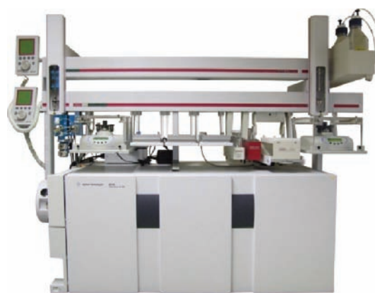
Figure 1. Anatune automated LC-QQQ system configured for online QuEChERS.
