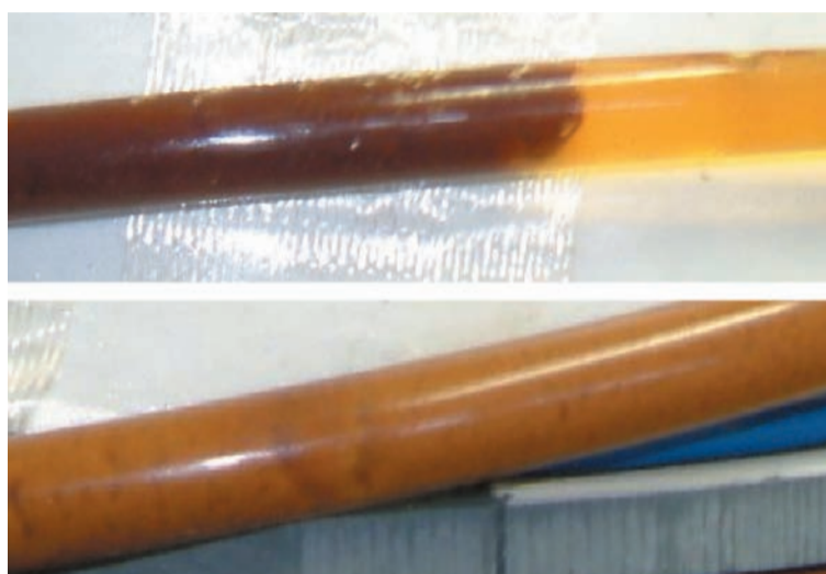
Figure 3. Two views of a sample loading tube reported in [8] showing particulate matter, which was subsequently successfully processed.
