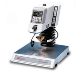
Figure 3: Digital Penetrometer [13].
