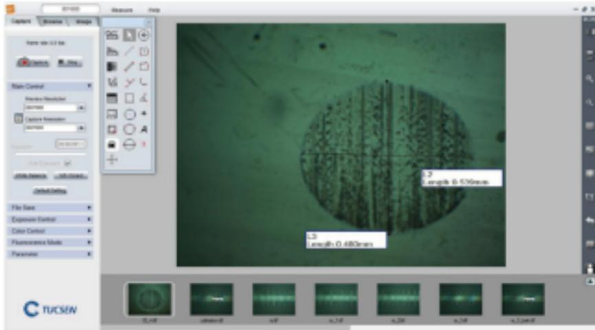
Figure 2: SEM imaging of wear scar after operation using K94190 BOCLE Lubricity Test rig.
