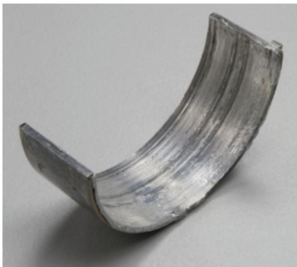
Figure 1. A spun-out connecting bearing from an automotive engine not being properly lubricated.
