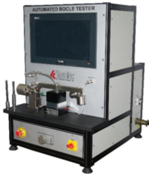
Figure 3: Image of the K94190 Lubricity Test Rig (BOCLE) by Koehler Instrument Co.
