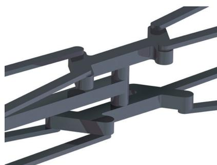
Figure 3. Flow channel example of a splitter in a mixer. The channel height is  $80\mu\text{m}$ .
