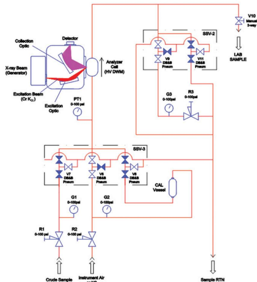
Figure 3 – Applied MWDXRF Process Analyser
