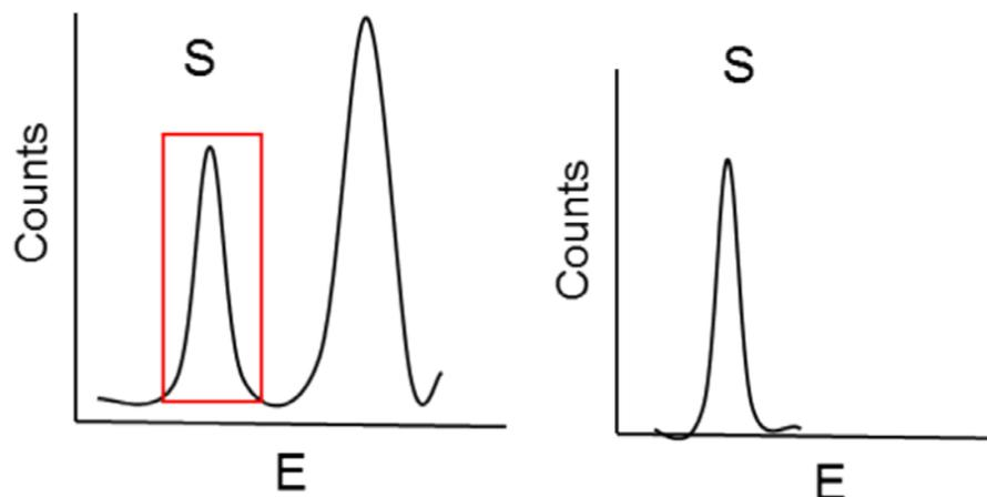
Figure 2 – (L) Sulphur Signal from sample excited by monochromatic excitation X-rays
