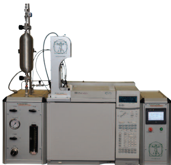
Figure 2: GC system dedicated to the Liquefied Gas Injector
