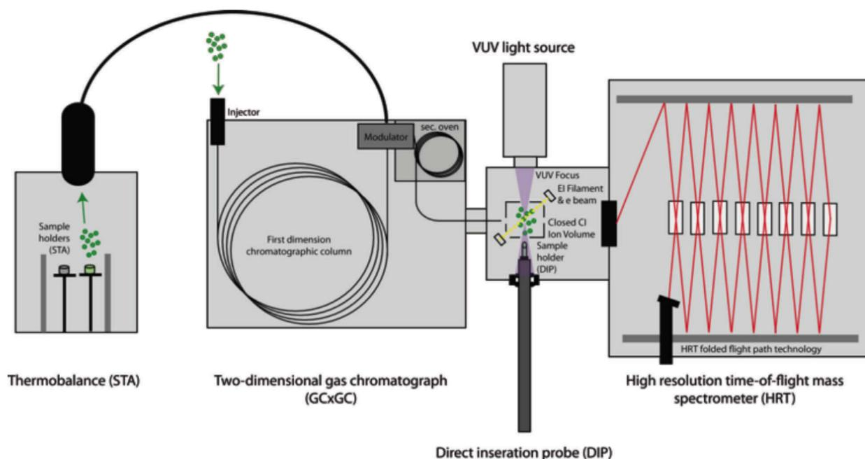
Figure 1: Schematic of a combined analytical system based on a LECO Pegasus GCxGC-HRT.
