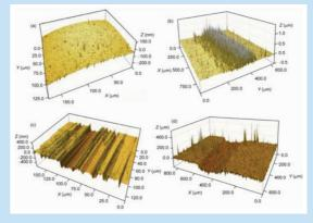
Figure 4. 3-D profiles of wear scar on the  $Si_3N_4$  ball (a) and the  $Al_2O_3$  plate (b) after friction experiment lubricated by GO colloid; 3-D profiles of wear scar on the  $Si_3N_4$  ball (c) and the  $Al_2O_3$  plate (d) after friction experiment lubricated by MD colloid.
