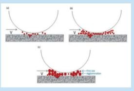
Figure 6. Lubricating mechanisms of TiO<sub>2</sub> at 0.2 %, 0.8 %, and 4.0 % (by weight).
