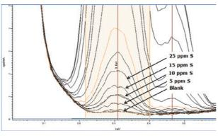
Figure 5: Overlaid sulfur signals in gasoline starting with a blank signal, followed by 5, 10, 15 and 25 ppm S. The integration range is shown in orange.
