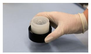
Figure 3: Liquid cup (Ø 40 mm) in SampleCare cup (Ø 51 mm). The liquid cup preparation tool can also be used to transport the sample from lab bench to measurement chamber.
