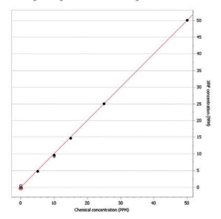
Figure 4: Calibration curve for sulfur in gasoline for the lower concentration
