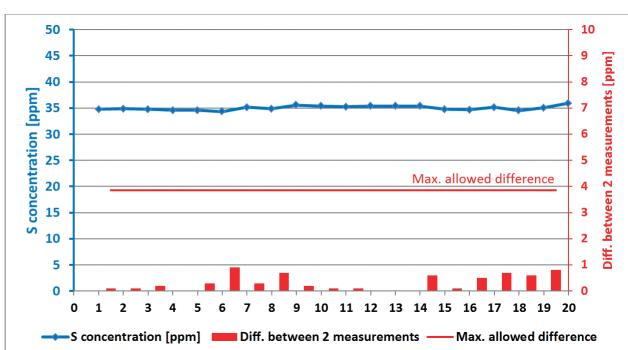
Figure 6: Repeatability of 20 measurements of a gasoline sample, according to ASTM D7220
