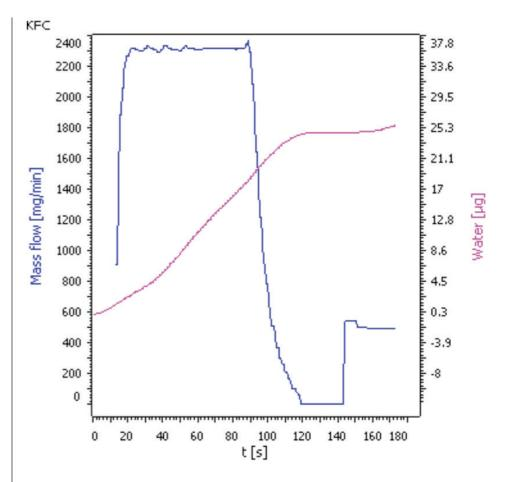
Figure 1: This typical curve of a Karl Fischer water determination in propane depicts the mass flow in blue and the amount of water that has been titrated in pink.
