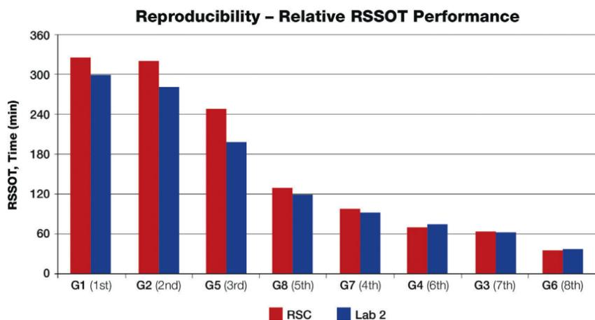
Figure 2: Studies concerning the reproducibility of the RapidOxy: Measuring the oxidation stability of 8 ELGI Rail WG 2012 RR greases in two different laboratories.
