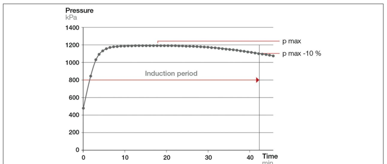
Figure 1: RSSOT / ASTM D7525 induction period - time elapsed between starting the heating procedure and a pressure drop of 10 % from the maximum pressure.
