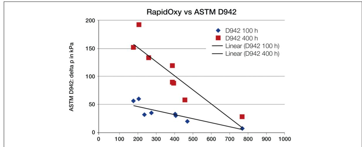
Figure 3: Correlation between the RapidOxy at 160 °C and ASTM D942 at 99 °C after 100 hours (blue spots) and 400 hours (red spots).
