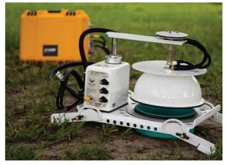
Soil gas exchange chambers are designed to minimize disturbance to the soil environment
