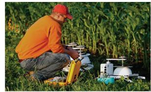
The LI-8100A system is ideal for measuring gas exchange from soils. It can be configured for single-chamber survey measurements or long-term measurements with up to 16 chambers.
