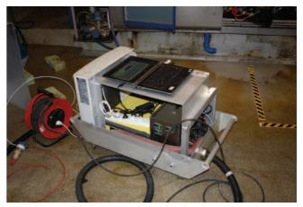
Gasmet's Danish Distributor C.K Environment A/S constructed a special cradle to protect the analyser and computer from the 'special conditions' inside a milking parlour
