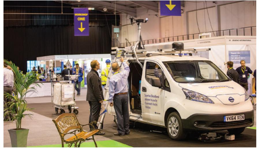
The demonstration area, featuring a "Monitoring on the Move" theme, included this van, equipped with a high speed multi-gas analyser
