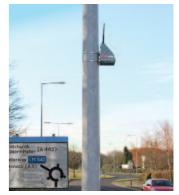
equipment can be conveniently positioned. The small postmounted units are completely wireless, using battery power and GPRS communications. AQMesh 'pods' measure the main air polluting gases and wirelessly communicate data to a 'cloud' where sophisticated data management generate highly accurate readings. Users can view or download data from up to hundreds of pods via an online portal.
