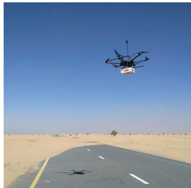
With a sensitivity over 1,000 times higher than conventional leak detection technologies, the OA-ICOS method permits the analyzer to detect single parts per billion (ppb) levels of methane and ethane every second, enabling variations in atmospheric concentrations to be quickly measured over long distances where other technologies would be ineffective.
