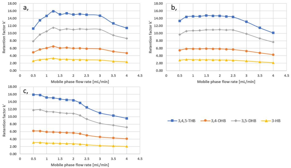
Figure 2: Retention dependency of mobile phase flow rate at different back pressure levels (a, 100 bar; b, 150 bar; c, 200 bar back pressure)
