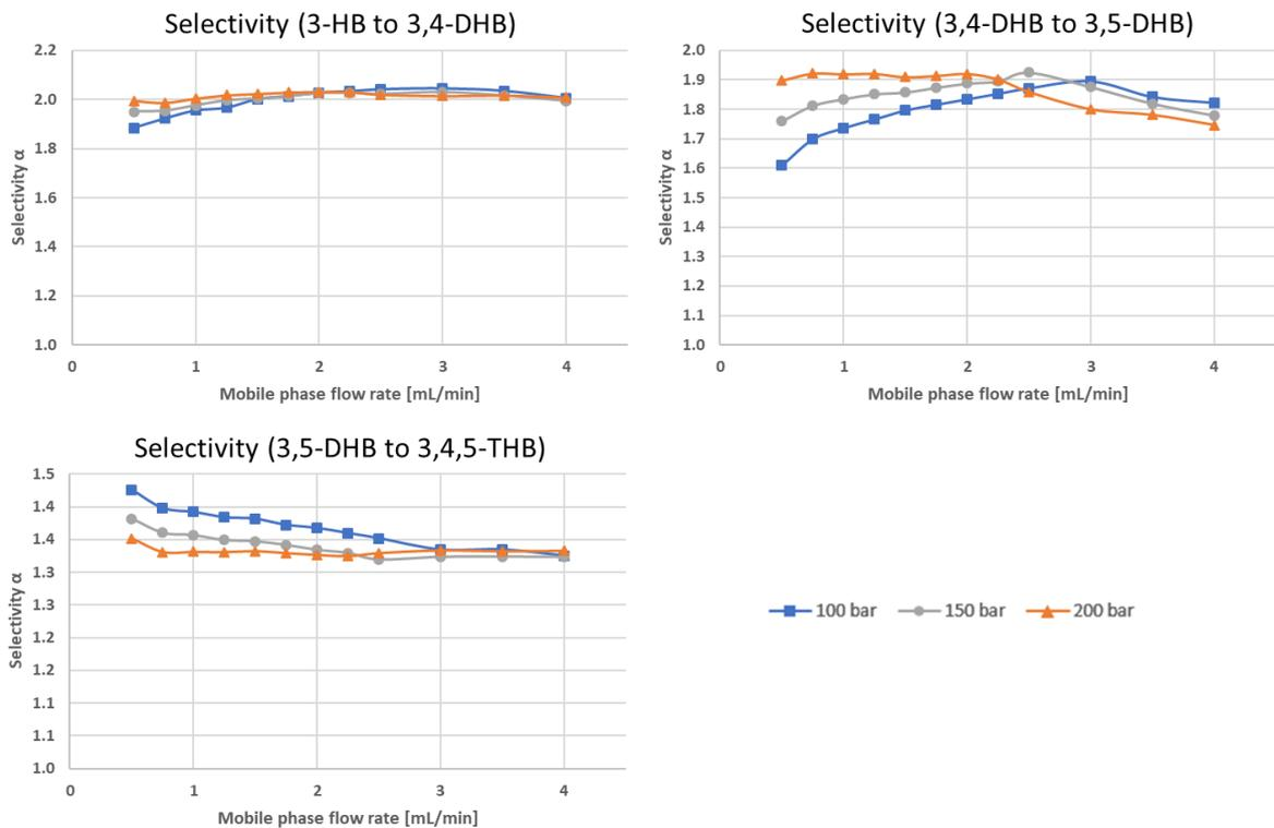
Figure 3: Selectivity dependency of mobile phase flow rate and back pressure level
