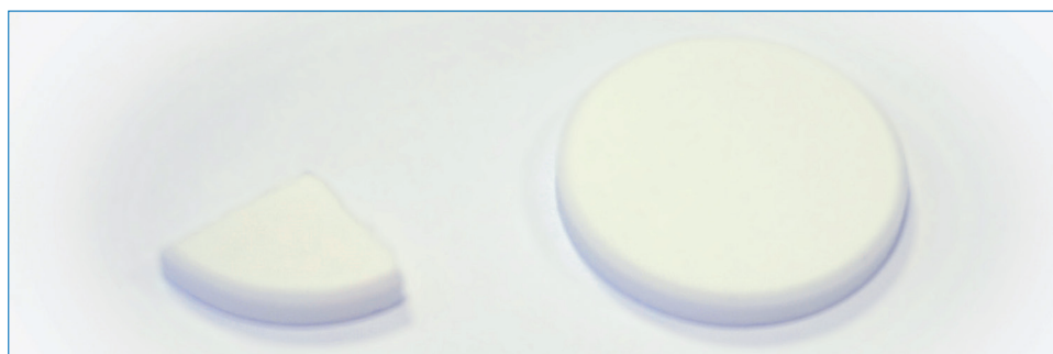
Figure 6: Upper surface of frits for inlet (left) compared to a new one (right).
