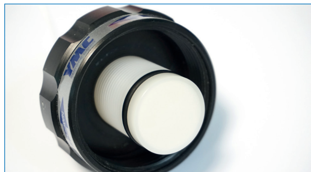
Figure 5: Outlet of the column after CIP method.
