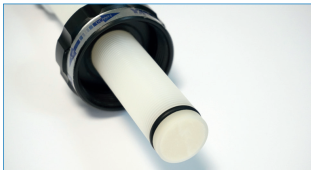
Figure 4: Inlet of the column after CIP method.
