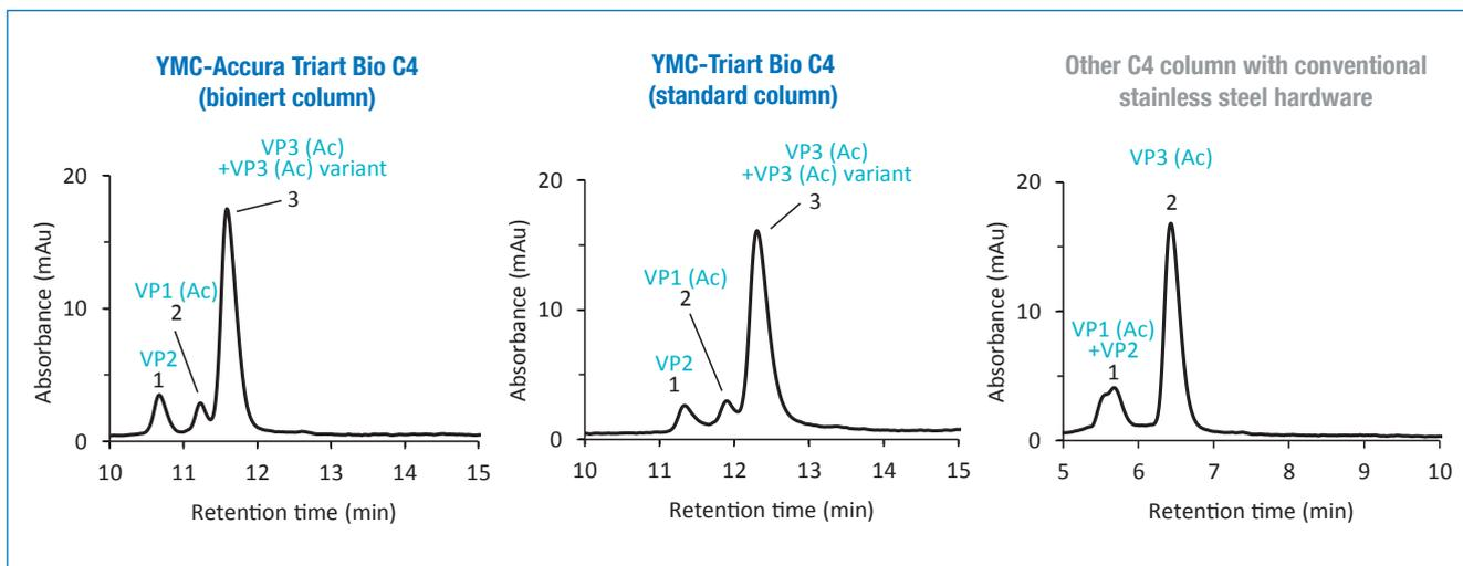
Figure 1: Comparison of VPs separation by RP-LC using the bioinert YMC-Accura Triart Bio C4, YMC-Triart C4 (standard hardware) and another C4 column with stainless steel hardware.
