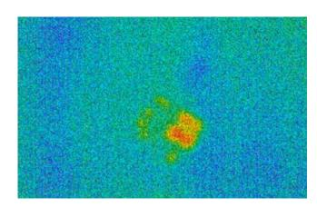
Uncooled thermal camera image of handprint on wall after 2 minutes
