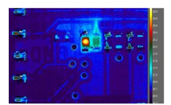
Uncooled thermal camera image of electronics board
