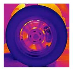
Uncooled Thermal Camera Image of Rotating Tire
