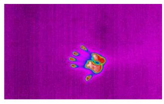
Uncooled thermal camera image of handprint on wall initial image
