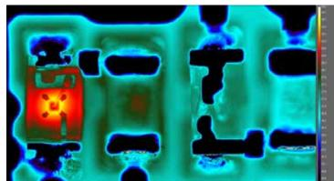
Cooled thermal camera image of electronics board
