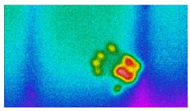
Cooled thermal camera image of handprint on wall after 2 minutes
