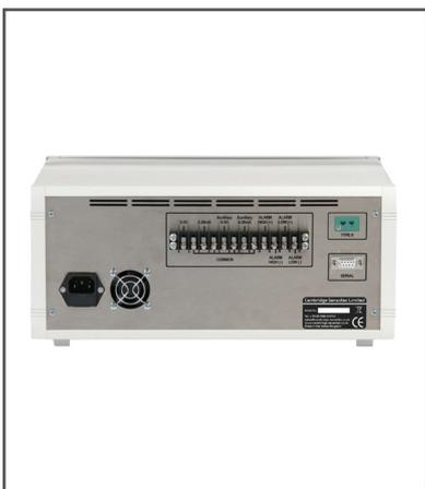
Standard features on all models include two fully programmable alarm circuits (voltage free contacts), programmable analogue outputs (0-10V and 4-20mA), easy calibration (user selectable gases), RS232 communications and complete data-logging software. Type K thermocouple input is included for independent temperature measurements up to 1250°C, with readings displayed and data logged simultaneously with the gas analysis.
