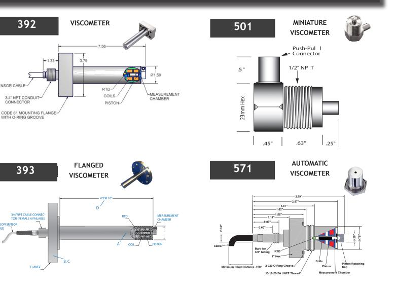
**Note:** Almost all process connections are available in both temperature options (low or high), all area classifications, and viscosity ranges (from 0.2 to 10,000cP). However, the 501 and 571 sensors are only available in the following options: low temperature, safe area hazard classification, and up to 500cP.
