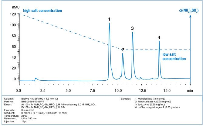
Figure 1: HIC analysis of four proteins using a decreasing salt gradient on a BioPro HIC BF column.
