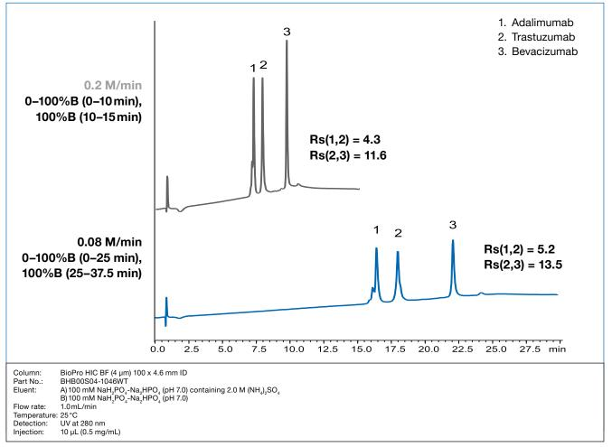
Figure 8: Separation of three mAbs using different gradient slopes.
