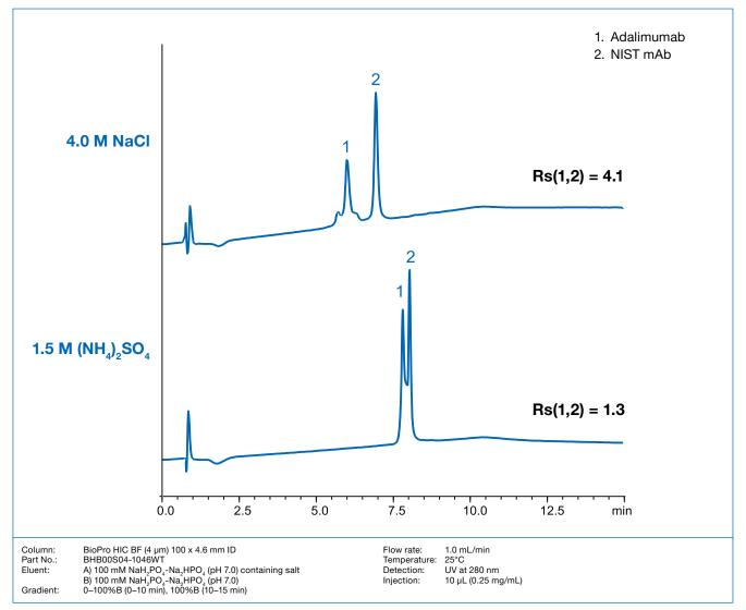
Figure 4: Separation of Adalimumab and NIST mAb using different type of salts.
