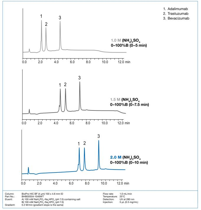
Figure 5: Separation of three mAbs using different initial concentrations of ammonium sulphate.
