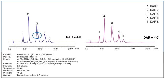
Figure 9: DAR analysis of brentuximab vedotin using 10 and 15% isopropanol as organic modifier.
