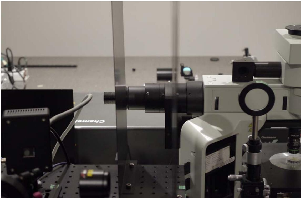
External view of two-photon excitation fluorescence microscope developed through our research
