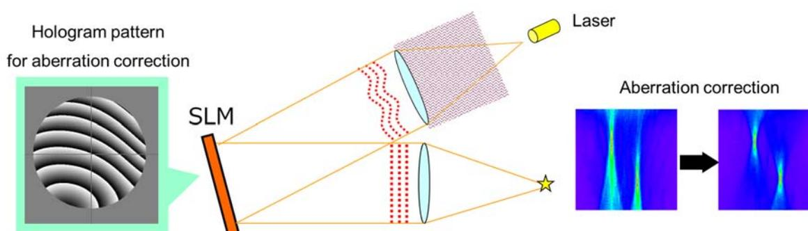
How SLM works to correct aberrations
