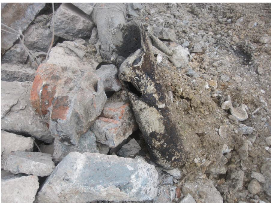
Crushed Chrysotile Bitumen Pipe
