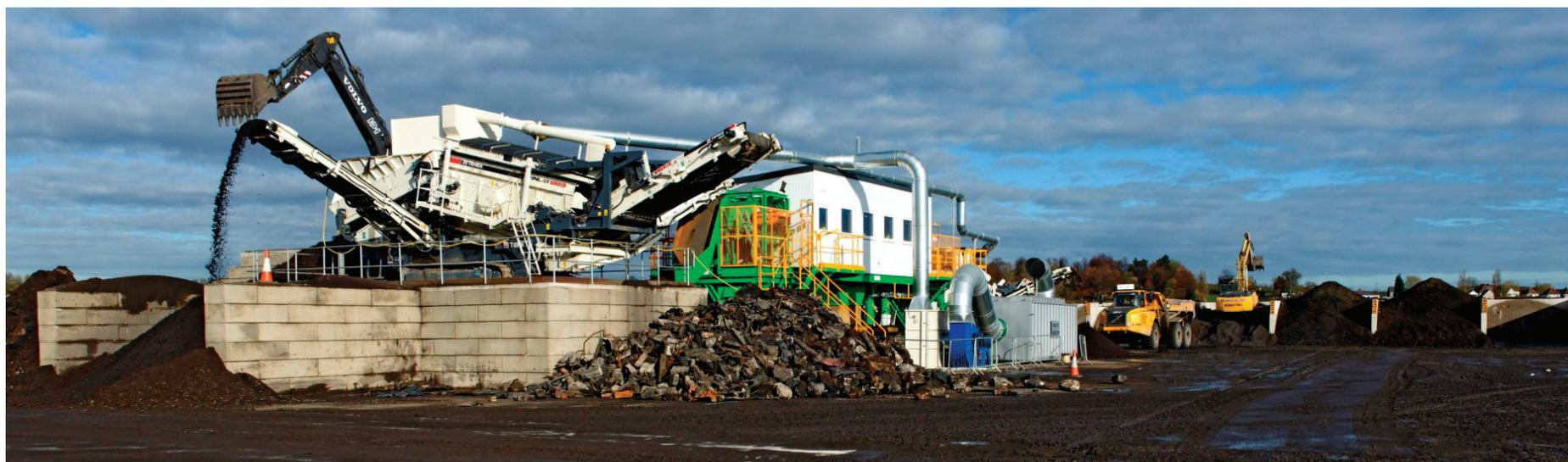
The excavation of the waste tip started in the summer of 2010 and around 327,000 m<sup>3</sup> of materials from the former licensed waste tip are being passed through the sorting process.
