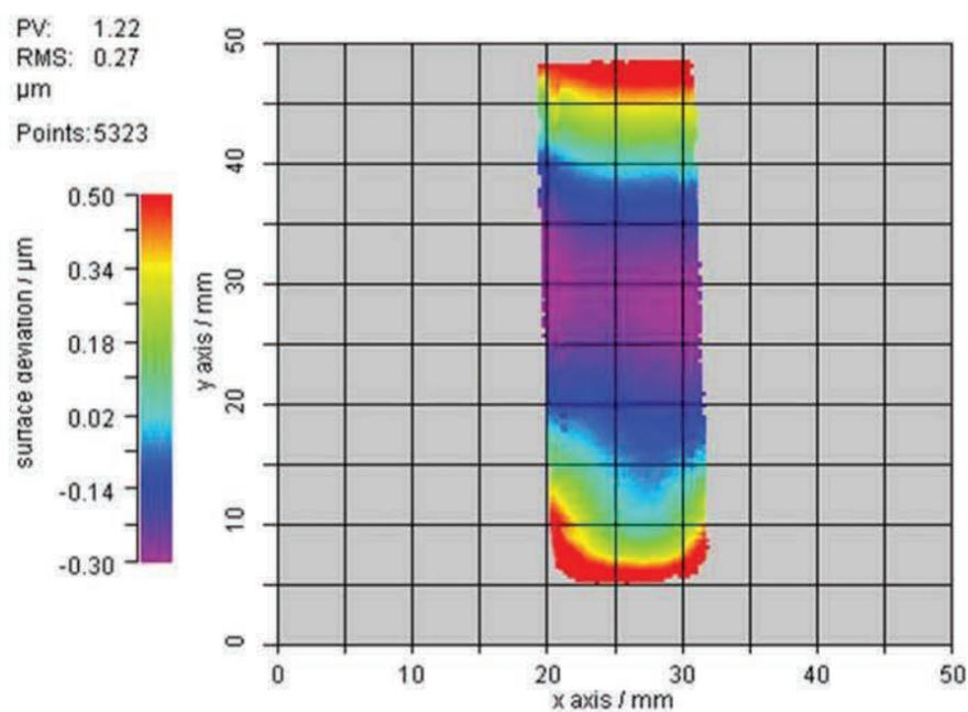
Figure 4 (b) surface scan of a lower quality cuvette
