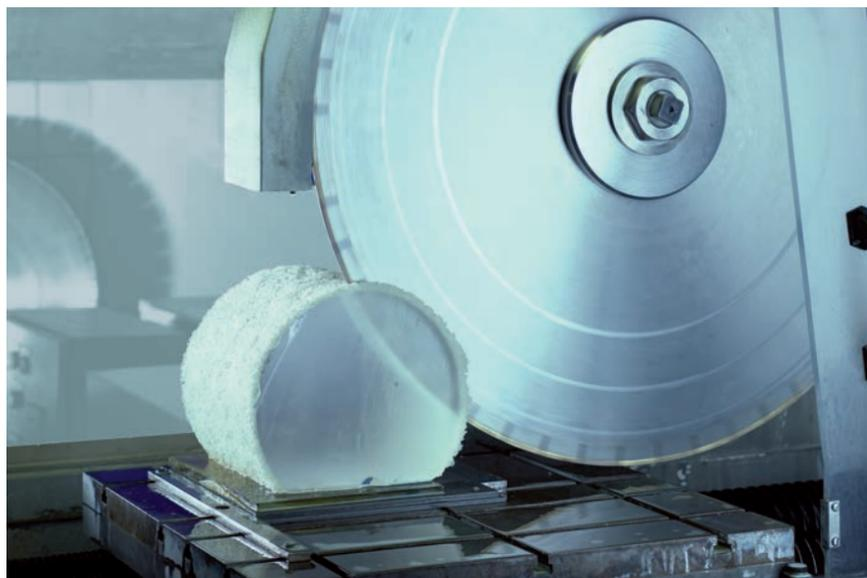
Figure 2: Cutting a block of Quartz to a workable size
