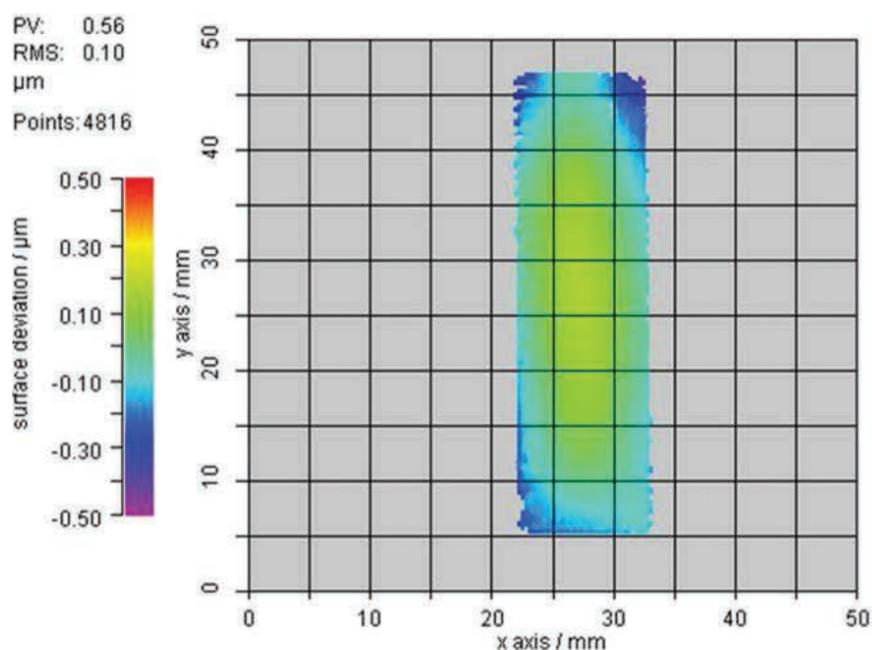
Figure 4 (a) surface scan of a quality cuvette
