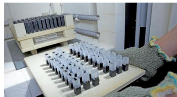
Figure 3: Cuvettes being stacked in an oven for the fusion process
