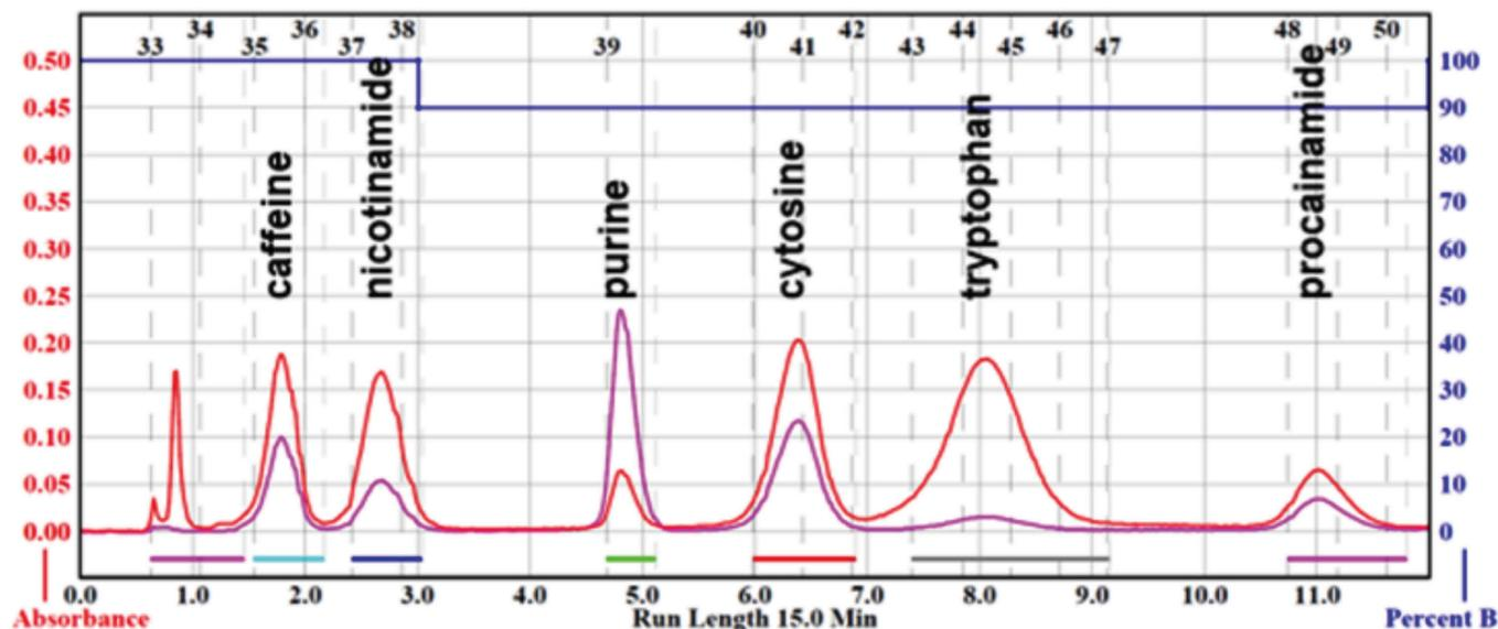
Figure 3. Flash Chromatography Polar Test Mix on 100-90% of B in A 3 min step gradient – Solvent A: Water with 10 mM ammonium formate; Solvent B: 95% ACN in water with 10mM ammonium formate; Teledyne ISCO 12g GOLD Silica (20-40  $\mu$ m) Redisep, 30 mlmin<sup>-1</sup>, 220 nm and 254 nm.
