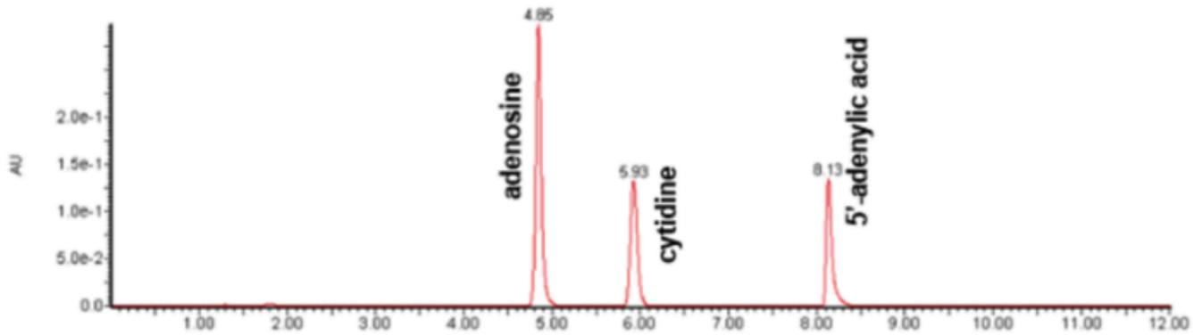
Figure 5. HILIC Analytical on 100-60% of B in A for 6 min gradient – Solvent A: Water with 10 mM ammonium formate; Solvent B: 95% ACN in water with 10mM ammonium formate; Atlantis HILIC Silica column 4.6x100mm, 5 $\mu$ m
