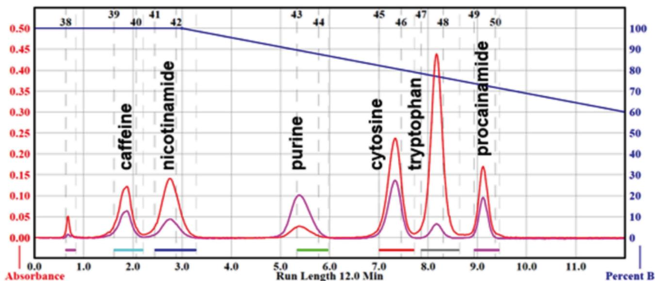
Figure 2. Flash Chromatography Polar Test Mix on 100-60% of B in A for 9 min gradient – Solvent A: water with 10 mM ammonium formate; Solvent B: 95% ACN in water with 10 mM ammonium formate; Teledyne ISCO 12g GOLD Silica (20-40 $\mu$ m) Redisep, 30 ml/min-1, 220 nm and 254 nm.
