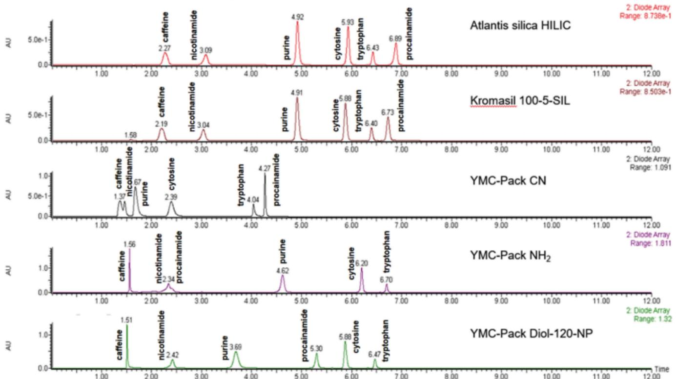
Figure 7. HILIC Analytical on 100-60% of B in A for 6 min gradient – Solvent A: Water with 10 mM ammonium formate; Solvent B: 95% ACN in water with 10mM ammonium formate;
