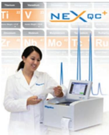
For more demanding applications, or for situations where analysis time or sample throughput is critical, **Rigaku** (USA) offers the new NEX QC+ spectrometer. Employing the next generation silicon detector technology, the enhanced NEX QC+ affords significant improvement in elemental peak resolution and counting statistics, resulting in superior calibrations and measurement precision for the most challenging measurements.
